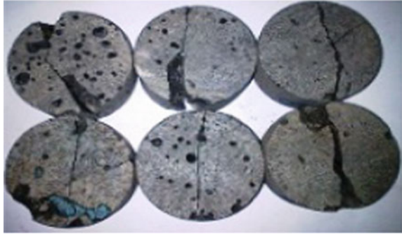
Fig. 10 Failure patterns of VB in Brazilian test
