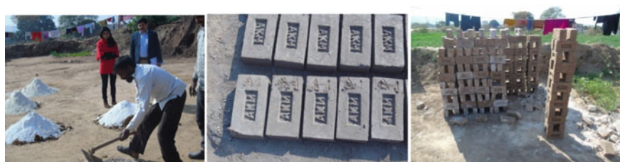
Fig. 1 Figures of bricks while mixing and formation (researcher getting the soil mixed with the sludge and thereafter formation of bricks out of it)
