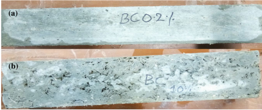
Fig. 1 Basalt fibre-reinforced concrete beam at a 0.2% and b 1% fibre content
